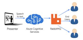
Above is the architecture diagram of the implemented solution. The presenter's speech is converted to text. The users are connected to the RabbitMQ server which places requests for the translated text and gives the response to the end users.
